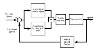
Fig. 3: Block diagram of typical automobile speed control system
