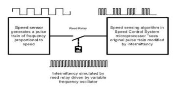
Fig. 5: Simulating the "false speed signal" effect with a reed relay
