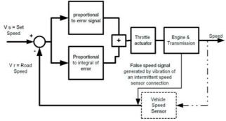
Fig. 6: Low speed operation of speed control system through agency of a false speed signal generated by a vibrating speed sensor connection
