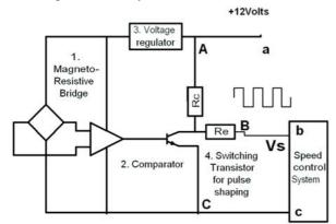
Fig. 4: A typical magneto-resistive speed sensor
