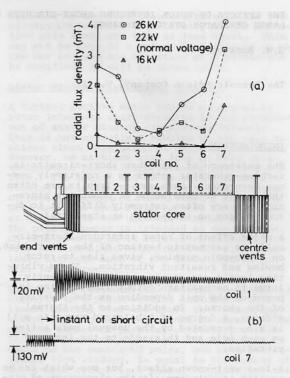
Figure 5 Flux density behind back of core on open circuit and search coil voltages during a sudden short circuit test
