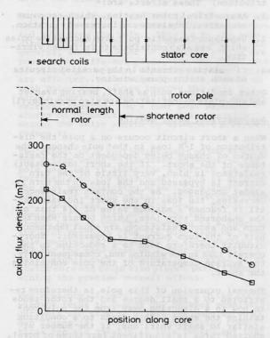
Figure 4 Axial flux density in stator teeth at normal open circuit voltage with normal and shortened rotor lengths
