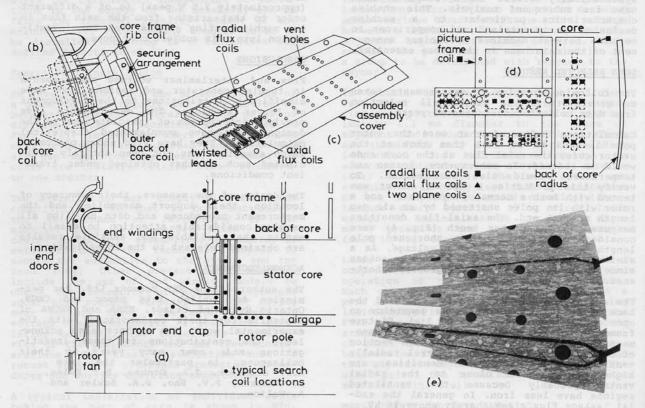
Figure 1 Sectional view of the end region of a generator, typical search coil locations and examples of assemblies
