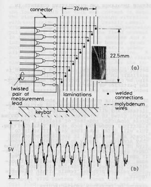
Figure 3 Connections of lamination voltage probes and an example of a 50 Hz interlaminar voltage wave
