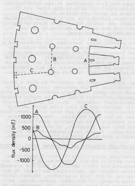
Figure 6 Radial and circumferential flux waves in a core section of a full scale model generator on open circuit
